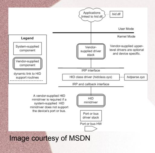
The HID device that the user mode applications or dlls is accessing is actually a class driver, or driver pair, which represents the underlying communications directly to the hardware.
