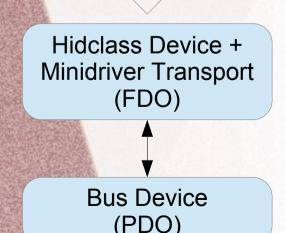
FDO : Function Device, Generally describes the device that talks UP the driver stack.
